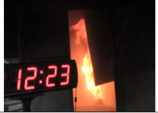
Figure 3. The sample on the right side of the ceiling began to fall off (12min:23s)
