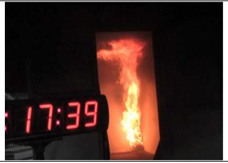
Figure 5. The sample on the left side of the ceiling began to fall off (17min:39s)
