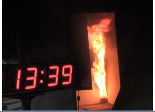
Figure 4. The sample in the middle of the ceiling a began to fall off (13min:39s)
